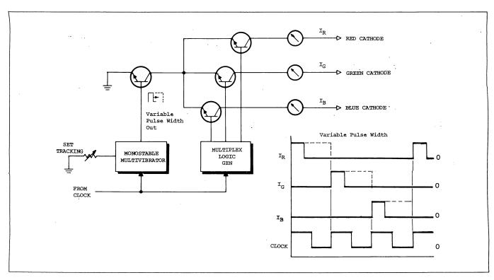
Fig. 8. Model 490 tracking test circuit (simplified).
